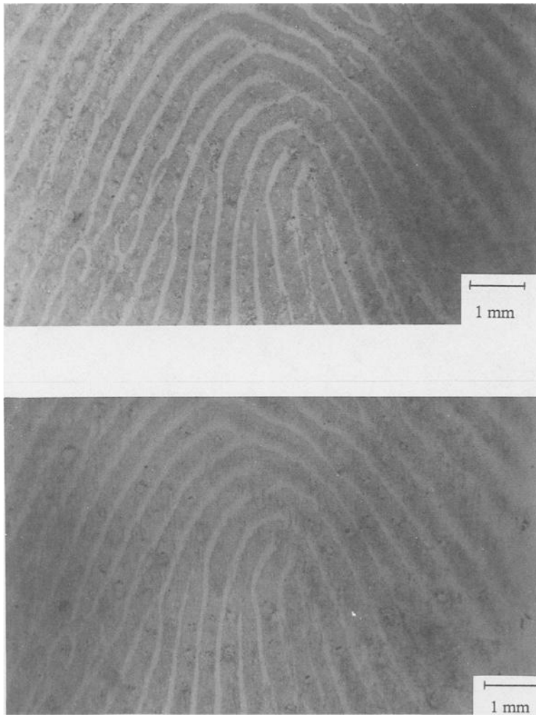
FIG. 3—Identical "standard" fingerprints: (top) as deposited; and (bottom) aged for 1 day, then brushed with 8 strokes of a clean squirrel-hair brush.
