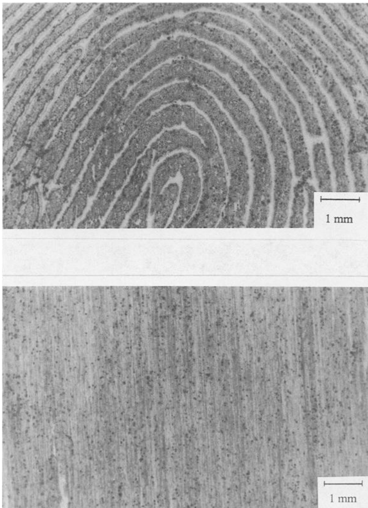
FIG. 4—Identical sebum-rich fingerprints: (top) as deposited; and (bottom) aged for 1 day, then brushed with 8 strokes of a clean squirrel-hair brush.
